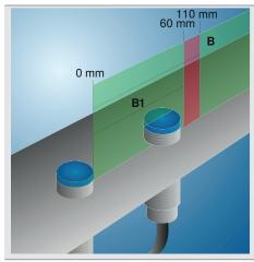
Example: B1 starts at 0 mm Installation B1 in mm: 0...60
