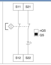
It is only permitted to connect safety solenoid switches to evaluation circuit SR4B3B01S if the requirements of standard EN 60947-5-3 have been met.
