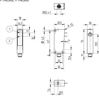
1 = emitter diode 2 = receiver diode
