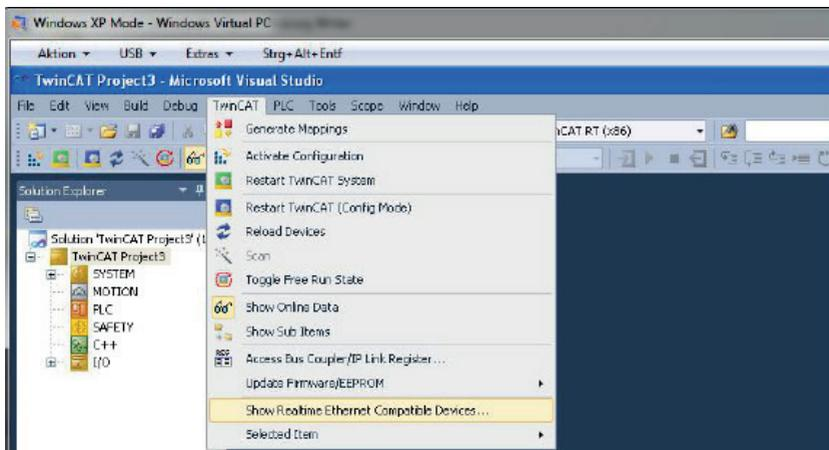
Incompatible network adapters can also be used for the connection. However, the performance will be different from compatible devices. A list of compatible realtime capable network adapters and current drivers can be viewed and/or downloaded on [www.beckhoff.de](http://www.beckhoff.de).
