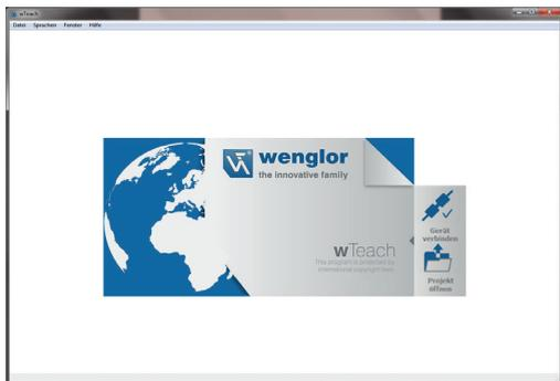
Before starting the program, it should be ensured that the sensor is connected to the computer. If the sensor is not connected until after the program has been started, the program has to be exited and restarted. After the program has been started, the following initial window appears and the software offers various options.
