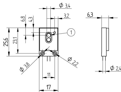
Maßangaben in mm/All dimensions in mm/Mesures en mm
