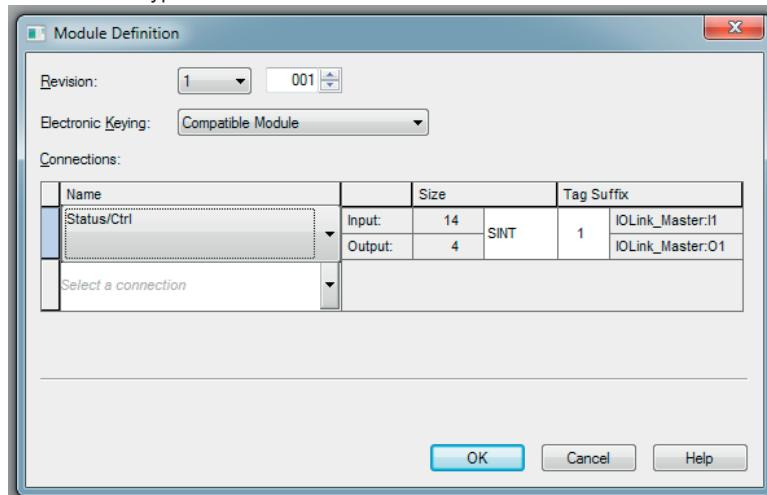
9. Select the type of connection. This selection determines which process data and diagnostics data will be made available by the IO-Link master.
