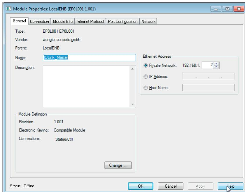
8. Click the “Change” button in order to change the settings for the module revision, electronic keying and connection type.
