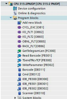
This is an overview of all of the blocks which are required for the use of scanner functions.
