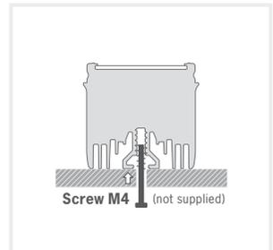
During the set up, the light has to be switched off and unplugged. Please use M4 screws and insert them in the captive nuts located in the back of the light. The light will be better fixed if you spread the attachment points symmetrically along the bar.
