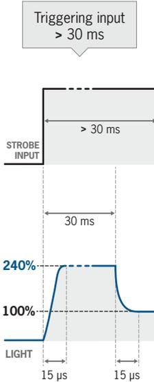
LED are supplied with 240% maximum current. After 30ms, LED are supplied at 100% level.
