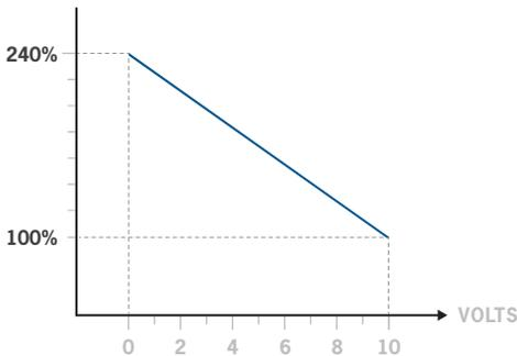
**Potential dimming between 0 & 10 V.**
