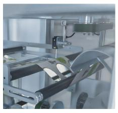
Print mark recognition to control various processes such as the alignment and positioning of objects or cutting, welding and gluing processes.
