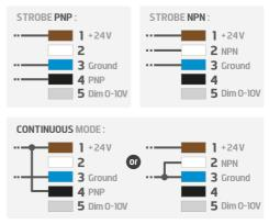
PNP: from 5 to 24V for 100% ON. From 0 to 1V for 100% OFF. NPN: less than 1V for 100% ON. Above 2V for 100% OFF. Max 20V.
