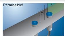
Two sensors can be mounted next to each other from installation dimension B.
