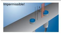
Two sensors must not be mounted in the area between B1 and R
