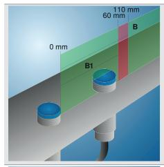
Example: B1 starts at 0 mm Installation B1 in mm: 0...60
