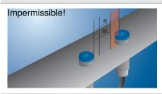
Two sensors must not be mounted in the area between B1 and R
