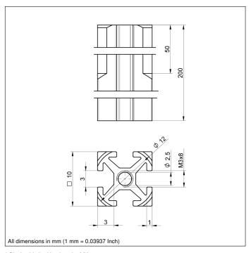
\* Single-sided, with a length of 50 mm trimmed off. The transition to a  $10\times10$  mm square has a chamfer of  $45^\circ$ .
