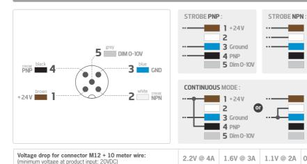
**EMC IMMUNITY CONNECTIONS:** for greater EMC immunity when using the light under Strobe operation, configure the signal connections as illustrated here. For Dimming, the Pin (5) should be connected to a voltage between 0V and 10V to ensure light output is correctly configured.
