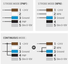
**EMC IMMUNITY CONNECTIONS:** for greater EMC immunity when using the light under Strobe operation, configure the signal connections as illustrated here. For Dimming, the Pin (5) should be connected to a voltage between OV and 10V to ensure light output is correctly configured.
