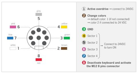
REMOTE CONTROL PINOUT THROUGH PNP: 0-4V is OFF and 5-24V is ON.
