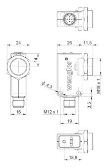
Dimensions in mm M3 screw = 0.5 Nm
