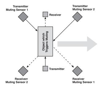
After muting has been activated as a result of obstruction of both muting sensors within a period of 4 seconds, the protective function of the safety field is deactivated.
