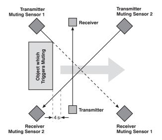
The muting sensors must be arranged such that both of their beams are obstructed by the object before it enters the safety field.
