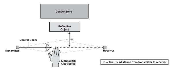
$\alpha$  = Opening Angle of Emitter and Receiver Optic
