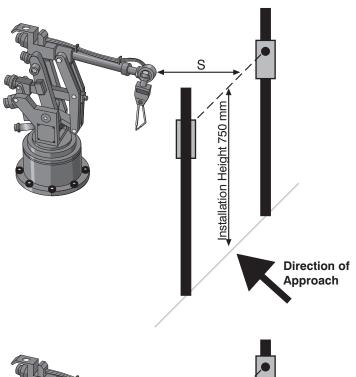
A minimum installation height of 750 mm from the reference level is required for the use of a light barrier
