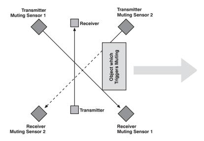
As soon as one of the muting sensors is no longer obstructed, muting is ended and the safety field is reactivated.
