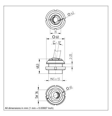
InoxSens is the hygiene series from wenglor. In addition to numerous other components, the InoxSens mounting console is also part of this complete system, which is seamlessly integrated into the machine. InoxSens sensors and mounting tubes can be fed through the system's side panel and mounted in a gapfree fashion with the help of the mounting console. Sensors can even be mounted to inclined surfaces, and can be quickly and easily adjusted thanks to angle compensation of up to 10°.
