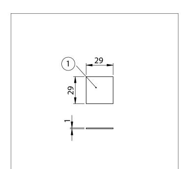
1 = Emitter and receiver side identical All dimensions in mm (1 mm = 0.03937 Inch)
