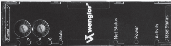
Picture 2: Front panel: Rotary switches and LEDs
