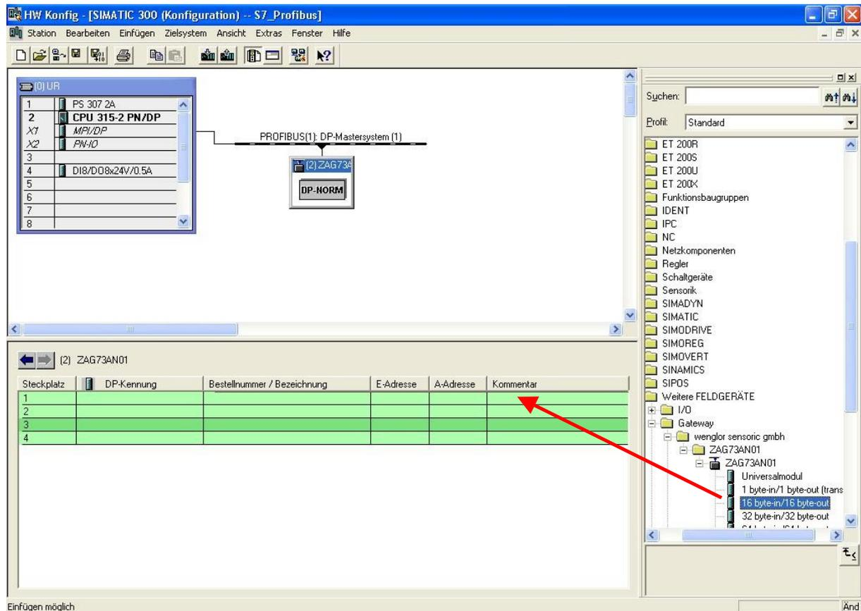
The screenshot shows the SIMATIC Manager HW Config interface. The main window displays a rack of modules (UR) and a Profibus DP-Mastersystem (1) connected to a ZAG73AN01 gateway. The table below the rack shows the DP list for the ZAG73AN01 gateway. The table has columns for Steckplatz, DP-Kennung, Bestellnummer / Bezeichnung, E-Adresse, A-Adresse, and Kommentar. A red arrow points from the 'Kommentar' column to the 'ZAG73AN01' gateway in the right-hand list of components.
