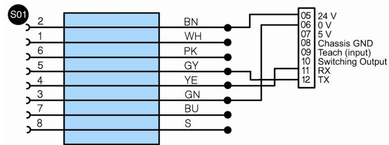
The sensor's switching output (e.g. A1) can be connected by wiring it to pin 10 at the gateway.
