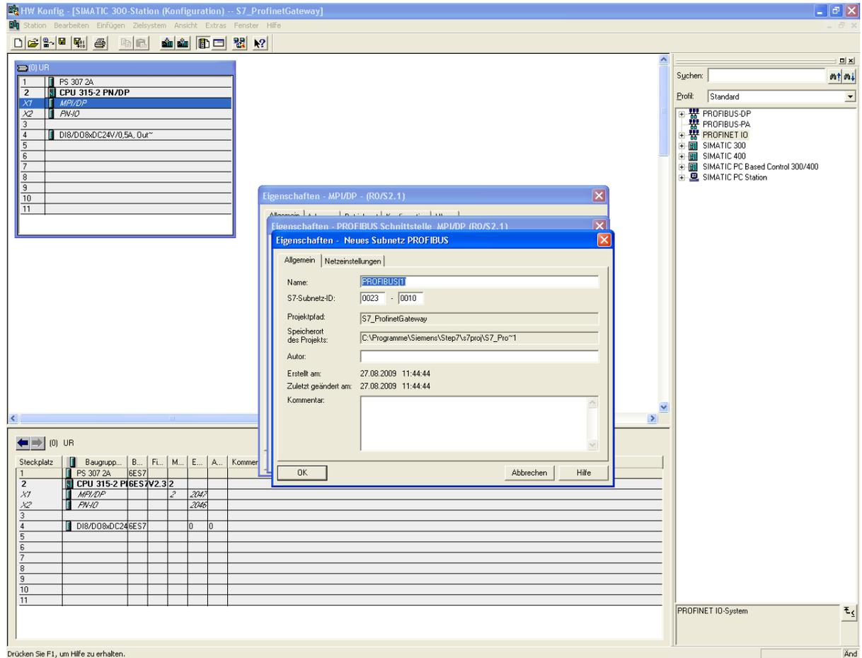
The screenshot shows the SIMATIC Manager HW Config interface. The main window displays a rack configuration for a SIMATIC 300 station. The rack is populated with the following components:
