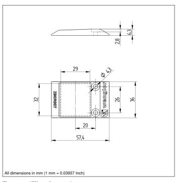
We recommend M4 mounting screws in accordance with DIN 960 for flush mounting.
