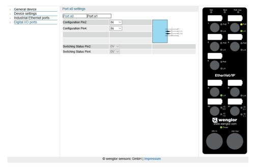
Pin 2 and pin 4 can each be configured as input or output. If the pin is configured as output, the pin can be set manually to 0 V or UB. A red flashing LED indicates a short-circuit on the respective pin.
