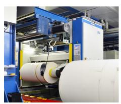
During the paper manufacturing process, OptoTemp sensors perform measurements at paper rollers and drying cylinders in order to monitor the drying process.
