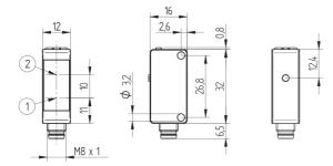
① = Emitter diode ② = Receiving diode Screw M3 = 0,5 Nm Dimensions specified in mm (1 mm = 0,03937 Inch)
