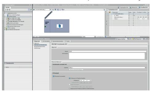
The screenshot above depicts a step-by-step procedure for changing the IP address of the OY2TA104P0150P sensor. The sensor is first of all accessed via the project tree. The sensor's properties window is activated by double clicking its icon (see screenshot above), after which the IP address can be set (see middle of screenshot).
