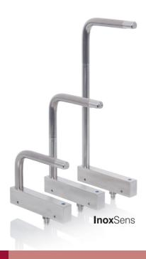
With fork widths of 50 to 220 mm, laser fork sensors offer new dimensions in flexibility and precision for quality control. They detect extremely small objects down to a size of 40  $\mu$ m at high process speeds of up to 10 kHz.
