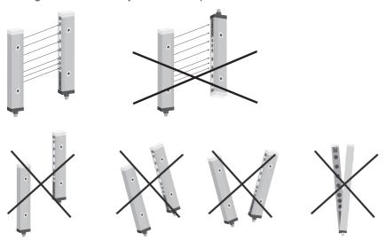
Correct alignment is indicated by the bar graph at the display. When all beams are shown as uninterrupted, the Light Barrier is correctly aligned.
