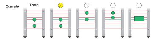
**Teach-In pattern, independent of position:** The taught in pattern can be located anywhere within the measuring field and is always recognized, thus causing the output to be switched.
