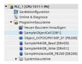
Overview of the blocks which are required in order to invoke (call) the teach-in function, the teach-in modes etc. of the OCPxxxP0150P sensor
