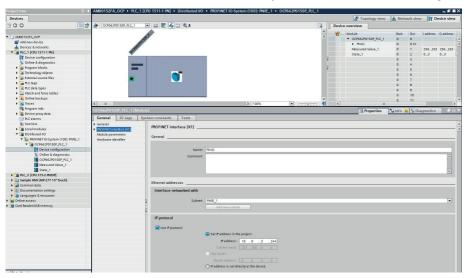
The screenshot above depicts a step-by-step procedure for changing the IP address of the OCPxxxP0150P sensor. The sensor is first of all accessed via the project tree. The sensor's properties window is activated by double clicking its icon (see screenshot above), after which the IP address can be set (see middle of screenshot at bottom).
