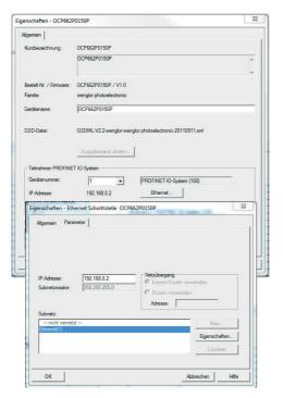
A menu window can be opened in the hardware configuration by double clicking the OCPxxxP0150P sensor. Amongst other settings, the IP address can be selected in this window.
