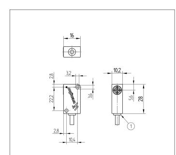
1 = Switching Status Indicator Screw M3 = 0,5 Nm All dimensions in mm (1 mm = 0.03937 Inch)
