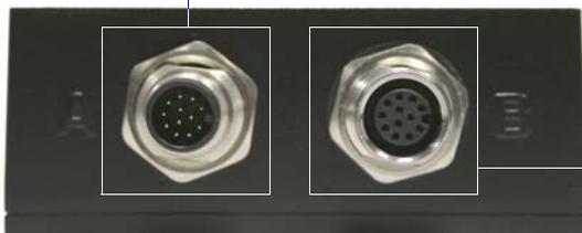
**Connector B** is a 12-pin socket on RS-232 scanner models, and an 8-pin socket on Ethernet models.
