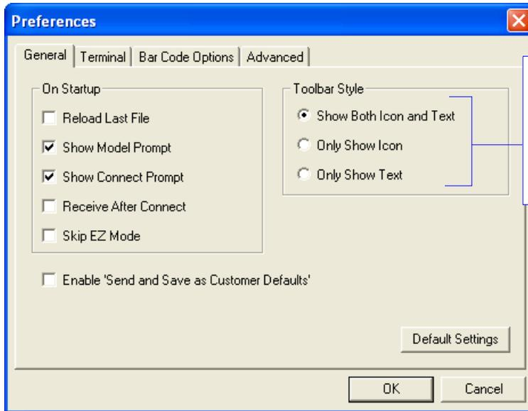
The **Toolbar Style** options allow the user to determine how **ESP** will display the mode options in the two rows at the top of the screen.
