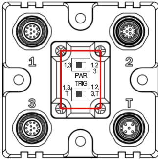
**Power** can be bussed between scanners and interface devices. At each location on a network where a new power supply is added, the Power switch on the AB-0830 can be used to break power between Connector 2 and Connectors 1, 3, and T.
