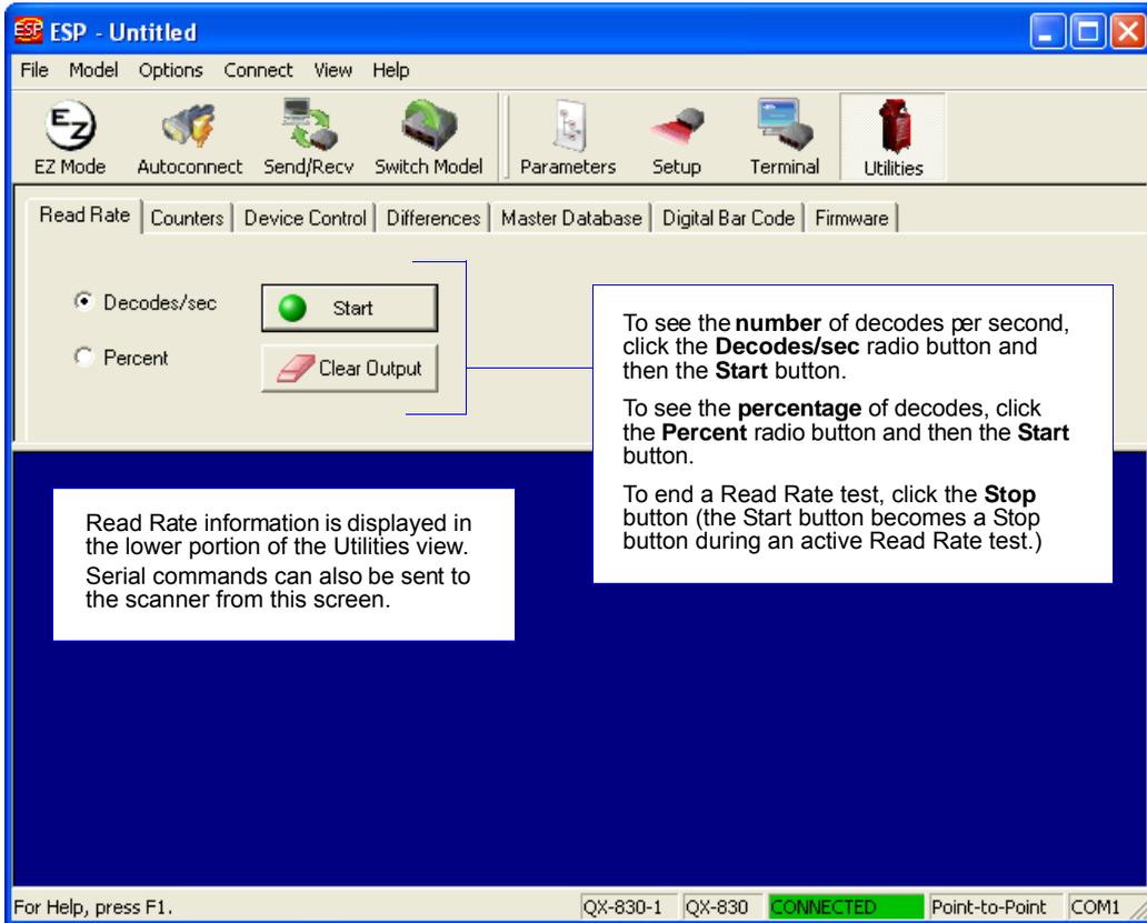
**Important:** When Read Rate is enabled, the **Configuration Database** is not active, regardless of how the scanner is configured.
