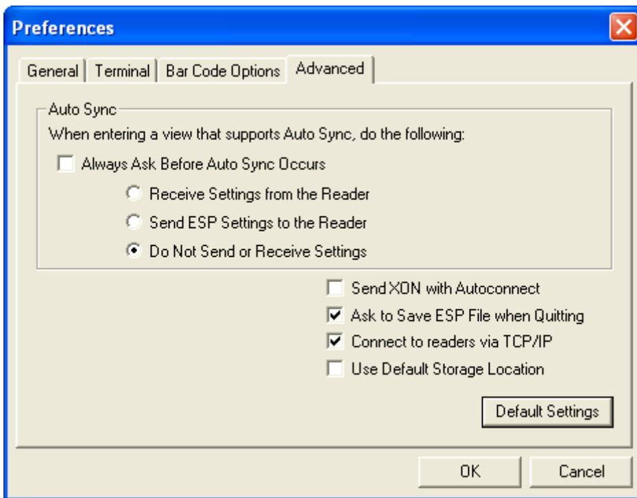
The **Auto Sync** options at the top of the **Advanced** tab allow the user to determine whether Auto Sync will be enabled automatically in sections of **ESP** where it is used, or if it will ask before it enables Auto Sync functions.
