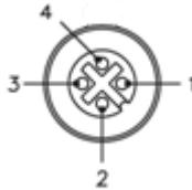
**AB-0830 Trigger Connector 4-pin Socket**
