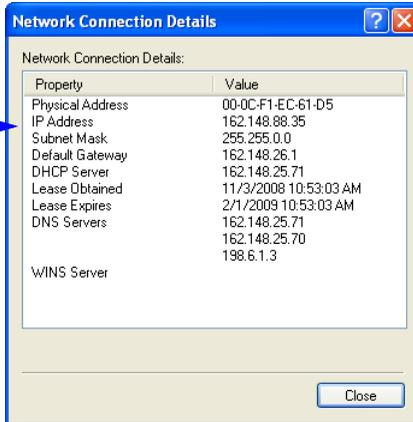
4. A connected FIS-0830's default address information can be verified in ESP by clicking the **Search** button in the **Connection Wizard**. Compare the scanner's IP address to the host's IP address to determine whether or not they are in the same range (this can be determined by your I.T. department if you are unsure).
