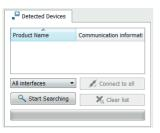
All sensors are searched for, detected and listed in the "Detected Devices" window along with the utilized interface.
