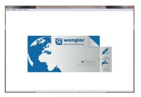
Before starting the program, it should be ensured that the sensor is connected to the computer. If the sensor is not connected until after the program has been started, the program has to be exited and restarted. After the program has been started, the following initial window appears and the software offers various options.
