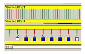
This object will be masked. The effected beams are selected to this end. The selected beams are highlighted in yellow, because the current configuration of the safety device differs from the configuration in the program.
