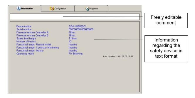
The most important data are listed as an overview in this window. All configuration files can be saved (\*.sst data file) or printed.
