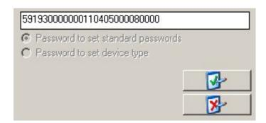
A code can be obtained from wenglor product support which allows the user to return passwords or the device type to their default settings (pass1, pass2, pass3).
