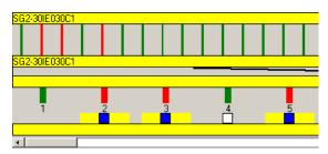
These objects will be masked. The effected beams are selected to this end. The selected beams are highlighted in yellow, because the current configuration of the safety device differs from the configuration in the program.
