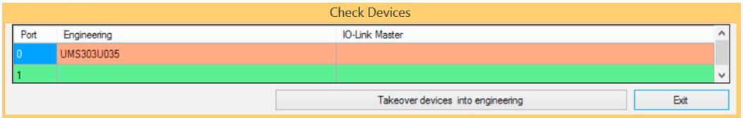
If an IO-Link device has already been added to the catalog, the device is detected and its name is displayed. Click Take over type of device into engineering in order to be able to configure the parameters of the IO-Link device
