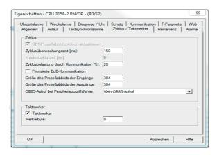
A menu window can be opened in the hardware configuration by double clicking the CPU. Amongst other settings, cycle flag bytes and the selection or deselection of the cycle flag can be implemented in this window.
