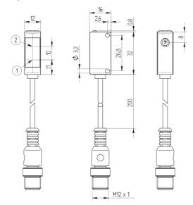
① = Emitter diode ② = Receiving diode Screw M3 = 0,5 Nm Potentiometer = 40 Nmm Dimensions specified in mm (1 mm = 0,03937 Inch)
