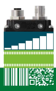
The scan software package transforms weQube into a 1D/2D code scanner for reliable decoding of even damaged or poorly readable codes by means of integrated code reconstruction.
