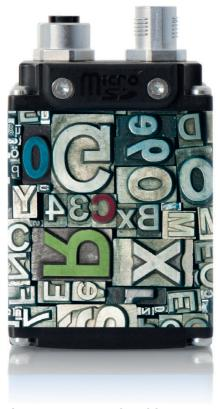
**Fonts:** weQubeOCR reads predefined OCR-A and OCR-B fonts over several lines in a single scanning operation.
