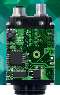
The **new weQube housing** with C mount threaded connection is compatible with all commercially available camera lenses based on the C mount standard. The great diversity of usable optics permits precise adaptation of the image to the respective application – for flexible ranges of vision from greater distances as well.
