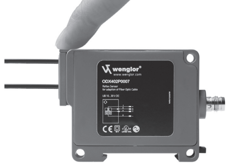
Fig. 8: Connecting the plastic fibre-optic cable
