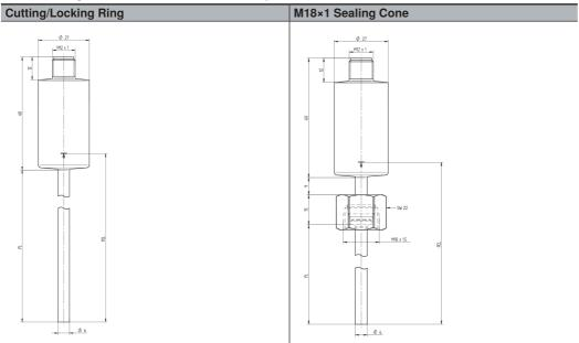
Process connection length PCL in the case of a cutting/locking ring = probe length PL + 9 mm Process connection length PCL in the case of an M18×1 sealing cone = probe length PL + 32 mm
