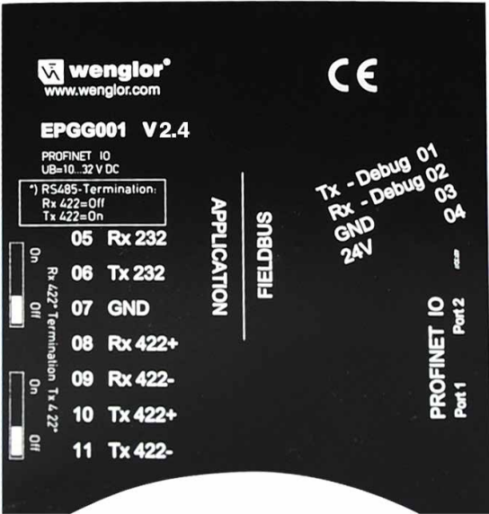
Figure 1: Connection labelling und termination
