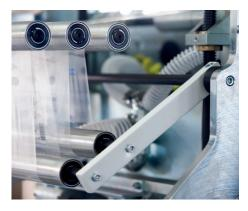
Packaging Industry In packaging processes, the reflex light barrier checks for the presence of transparent packaging materials, for example cellophane and blister packs.
