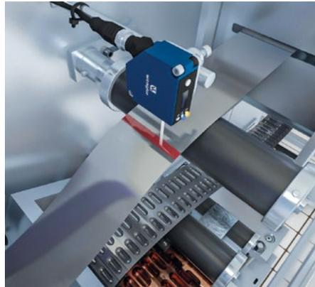
▼ **Check the material end** via visual marks, for example to initiate a timely roll change of film material.
