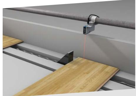
**Woodworking Industry** When producing prefabricated parquet floors, high-precision laser distance sensors ensure that the assembled wood layers are applied precisely in the correct position. Sensors with analog output are used to accurately detect the different heights of the individual parquet layers.
