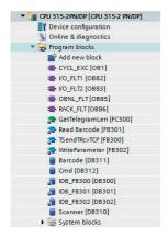
This is an overview of all of the blocks which are required for the use of scanner functions.
