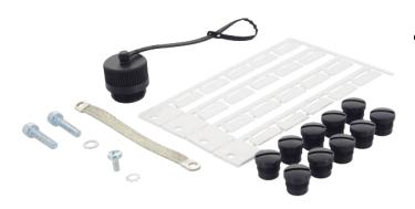
Content: 1 × 4,3 mm toothed lock washer, 1 × 4 mm² grounded flat plug connector, 1 × M4 × 8 mm screw, 2 × M5 × 20 mm screws, 2 × washers, 1 × rating plate set (20 plates), 10 × M12 screw-in plugs, 1 × 7/8" cover cap
