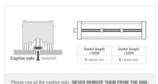
During the set up, the light has to be switched off and unplugged. Please use M4 screws and insert them in the captive nuts located in the back of the light. The light will be better fixed if you spread the attachment points symmetrically along the bar.
