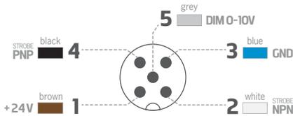
The **M12 male connector 5 points** is **COMPLIANT** with the M12 female connector 4 points. In that case, the dimming option is not available.
