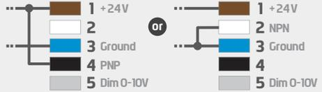
**EMC IMMUNITY CONNECTIONS:** for greater EMC immunity when using the light under Strobe operation, configure the signal connections as illustrated here. For Dimming, the Pin (5) should be connected to a voltage between 0V and 10V to ensure light output is correctly configured.
